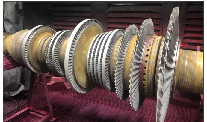
Steam Turbine Rotor
